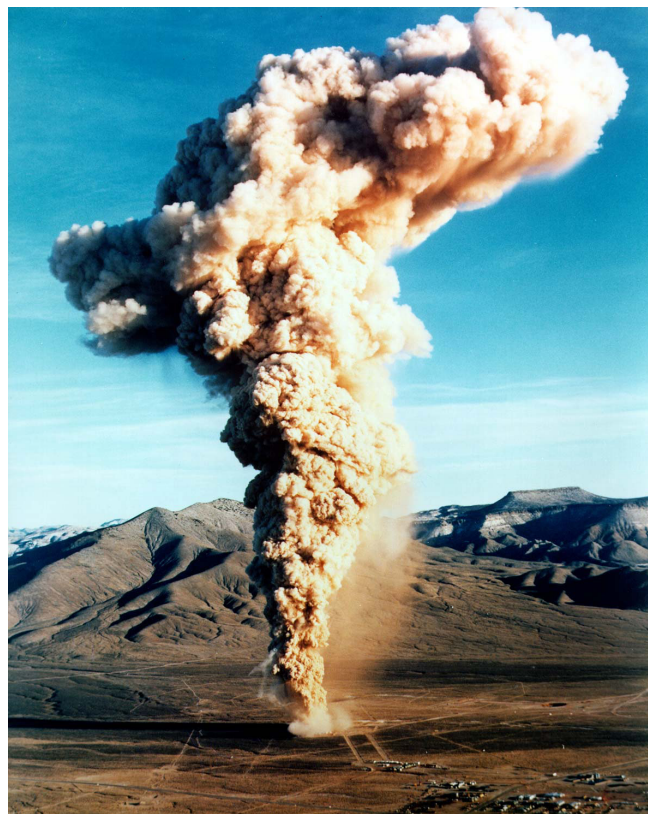
Figure 13. 1970 Baneberry Event Venting through Undetected Rock Fissure
