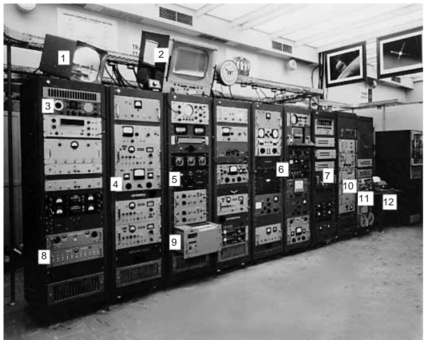
Figure 1. Experimental tracking station at APL (1962): 1 = antenna monitor, 2 = spectrum display, 3 = WWV (call letters) receiver, 4 = receivers and tracking filters, 5 = antenna positioner, 6 = meters, 7 = transistorized digital data system, 8 = refraction correction unit, 9 = recorder, 10 = antenna time recovery system, 11 = satellite time recovery system, and 12 = PB-250 computer.
