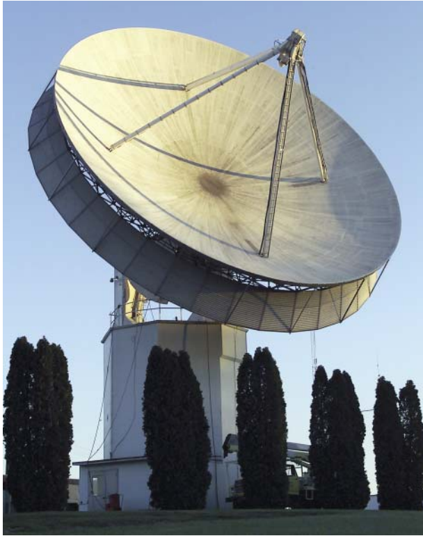
Figure 6. The APL 60-ft antenna is remotely controlled from the SCF. It is the primary antenna used to control the TIMED spacecraft.
