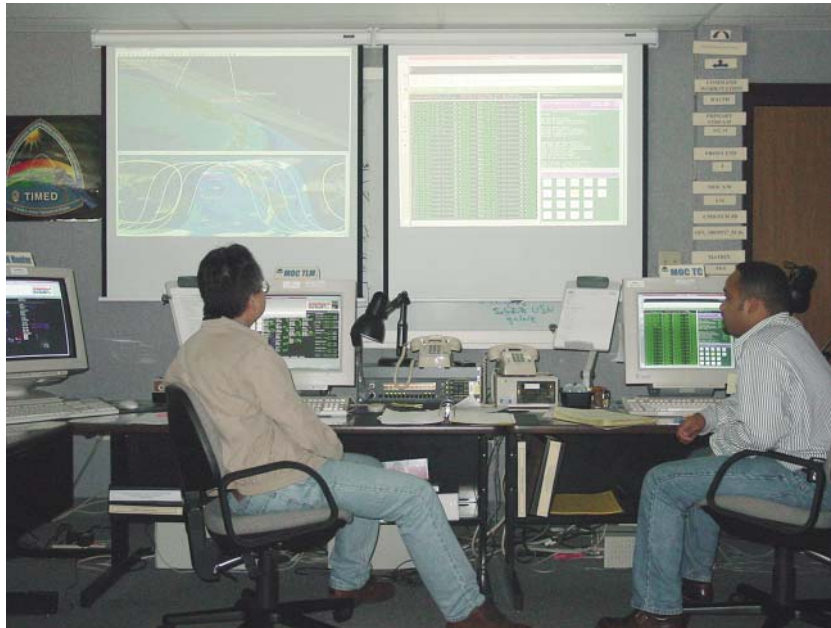
Figure 3. The TIMED MOC. The primary and backup command workstations are viewed by two of the TIMED Mission Operations Team members. The overhead displays are used to project spacecraft ground track, real-time attitude state, and spacecraft house-keeping data.
