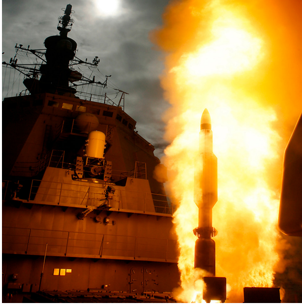
Figure 7. USS Lake Erie (CG 70) launching the Standard Missile-3, which intercepted the satellite during the Burnt Frost mission. The missile struck a nonfunctioning US satellite as it traveled in space at more than 17,000 miles per hour over the Pacific Ocean. The nation called on APL, with its long experience with Aegis and Standard Missile, to make vital contributions to this critical operation. (US Navy image.)
