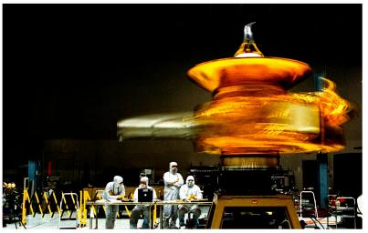
Time-elapsed photo of the spacecraft spin balance test at NASA Goddard Space Flight Center in June 2005.
