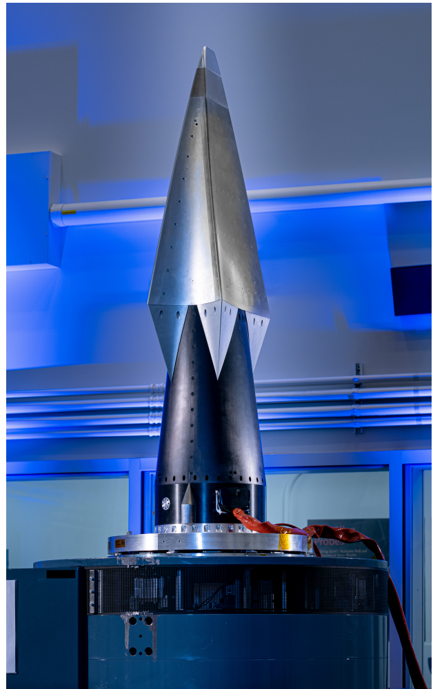
Figure 10. The completed BOLT flight experiment payload undergoing vibration testing at APL's Environmental Test Facilities. During testing, which included vibration and thermal testing over 2 weeks, sensors and electronics performed well during testing. All operational sensors remained responsive after testing.
