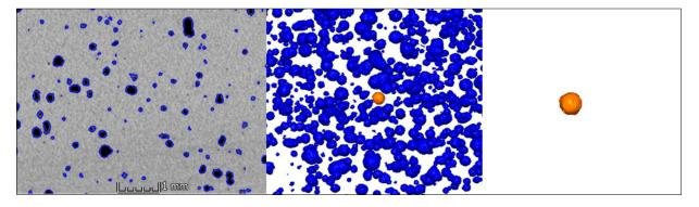
**Figure 2.** XRCT data processing techniques for identification of porosity in an AlSi<sub>10</sub>Mg AM specimen. The defect structure is seen in the 2-D slice (left) and can be segmented in 3-D (middle) and uniquely quantified (right).
