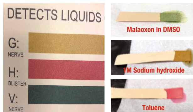
Figure 3. M8 paper, commonly used in the field for chemical agent detection. Shown are the standard M8 paper color key (left) and false positive results of M8 paper with common chemicals (right).
