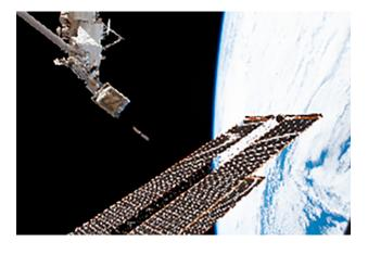
**Figure 5.** CAT (CubeSat Assessment and Test) being deployed from the ISS. Each of the two CubeSats in this APL-led flight demonstration carries a communications payload that was integrated by APL.
