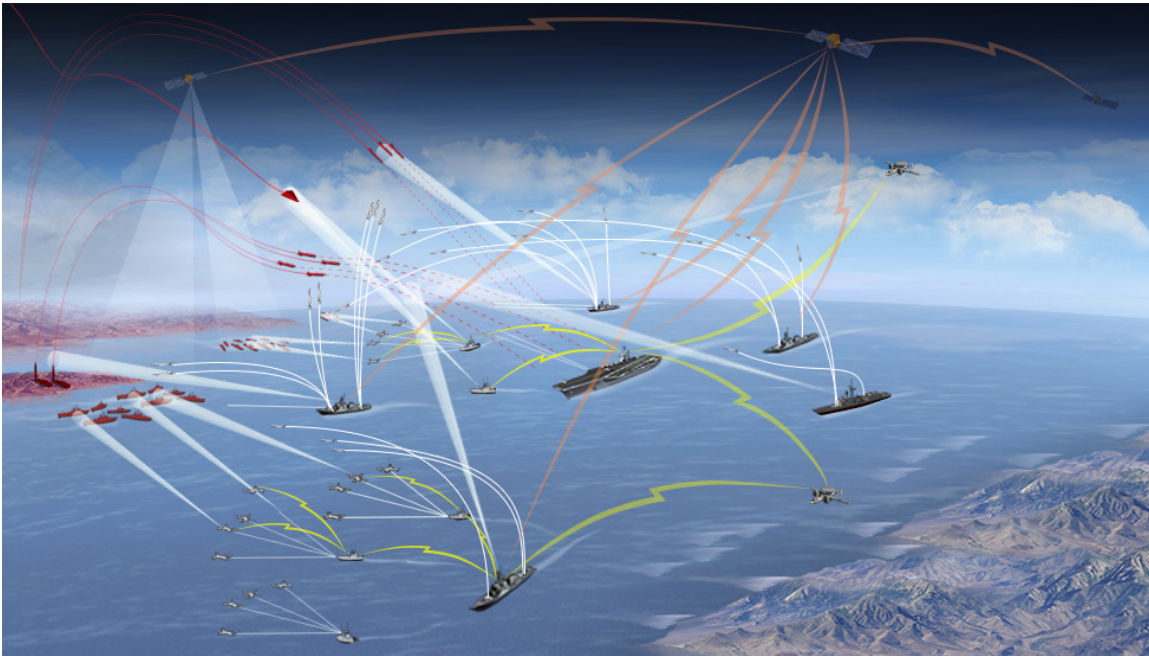
Figure 2. Envisioned kill webs enabled by ubiquitous ISR&T. Composable networks of space-based sensors (satellites), manned and unmanned surface and airborne sensors, and ground sensors are envisioned to enable adaptable targeting across air, surface, and ground threats.
