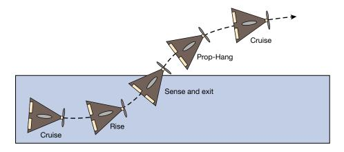
**Figure 4.** Diagram of flight behavior during a water-exit maneuver. Real-time state estimation is used to detect the transition point as the vehicle exits the water.
