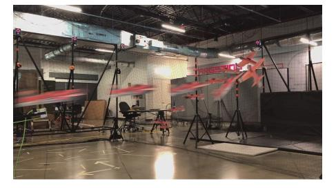
Figure 2. Time-lapse image showing a small fixed-wing aircraft performing a sharp 90° turn.
