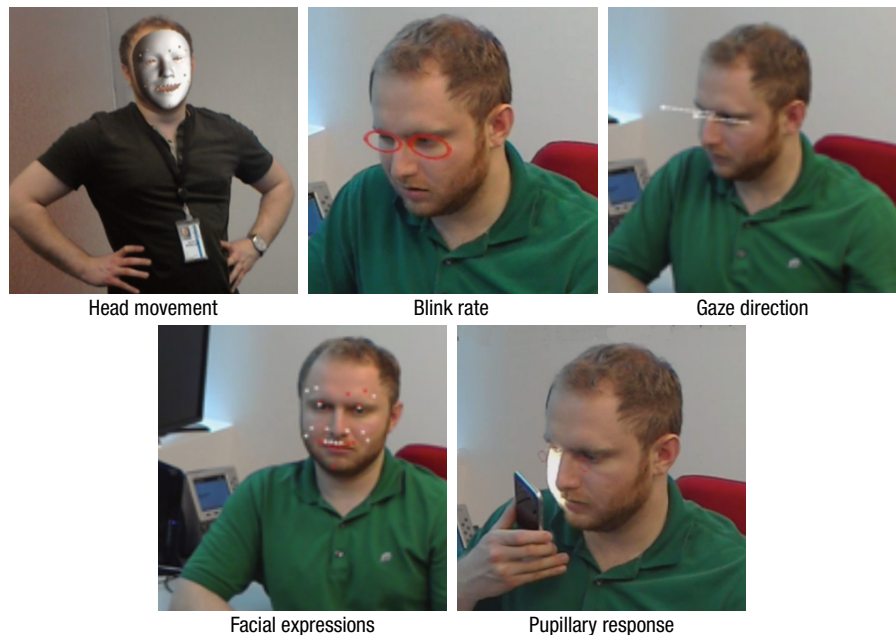
Figure 3. The MR social prosthesis system enables finer perception of nonverbal cues. The interviewer wearing the headset is able to view data points overlaid on the interaction partner's face, enabling the wearer to receive information in a way that is easily interpretable, in real time, and without interrupting the social interaction.
