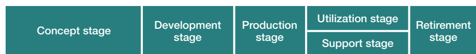
Figure 4. INCOSE generic development life cycle. This is a basic systems engineering life cycle for system development. 3
