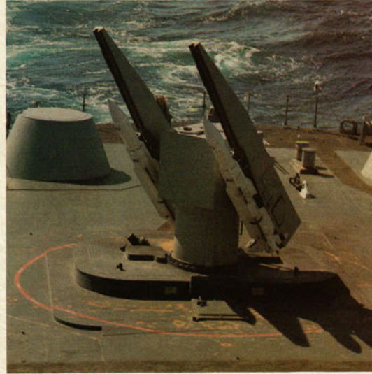
Figure 6 — STANDARD Missile is fired from dual rail launchers. The Mk 10 launcher fires the extended-range version from TERRIER ships while the Mk 26 launcher fires the medium-range version from TARTAR and AEGIS ships. Missiles are loaded horizontally onto the Mk 10 launcher and vertically onto the Mk 26 launcher.
