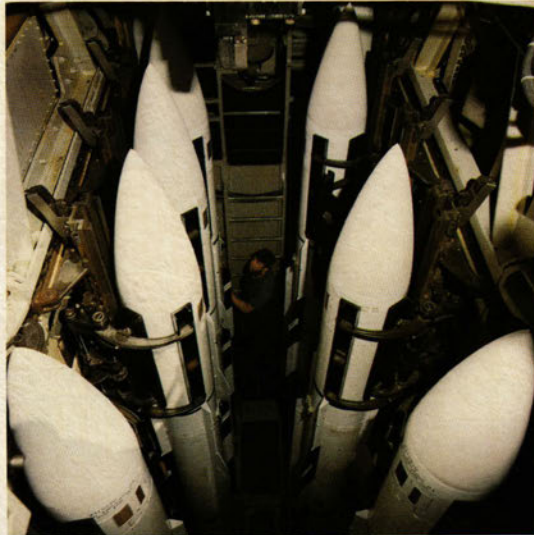
Figure 6 — STANDARD Missile is fired from dual rail launchers. The Mk 10 launcher fires the extended-range version from TERRIER ships while the Mk 26 launcher fires the medium-range version from TARTAR and AEGIS ships. Missiles are loaded horizontally onto the Mk 10 launcher and vertically onto the Mk 26 launcher.
