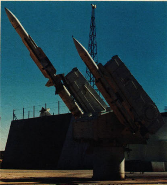
Figure 3 — TERRIER and TARTAR Missiles on launcher at White Sands Missile Range. The extended-range TERRIER Missile has a separate booster.
