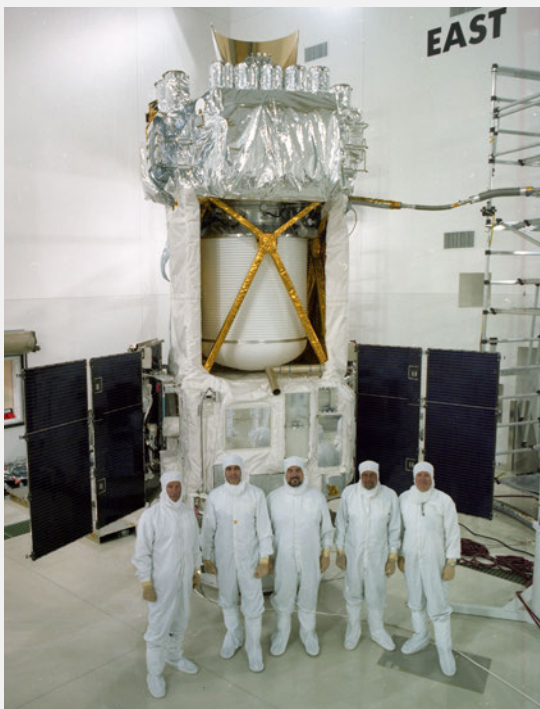
Figure 2. The MSX spacecraft, carrying the first-ever solid hydrogen IR detector cooling system launched into space, in fully tested flight configuration.
