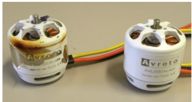
Figure 2. Motor treated with corrosion-resistant coatings (right) and control (left, untreated) after both were immersed in salt water for 8 weeks.
