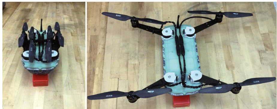
Figure 13. Folding CRACUNS platform model showing folding arms for stowage inside an unmanned underwater vehicle.
