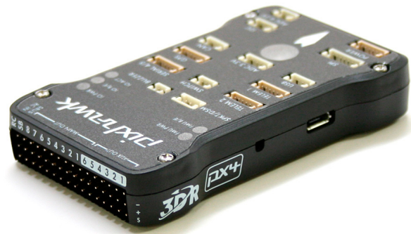
Figure 3. Pixhawk commercially available open-source autopilot. (Image from https://pixhawk.org/modules/pixhawk .)
