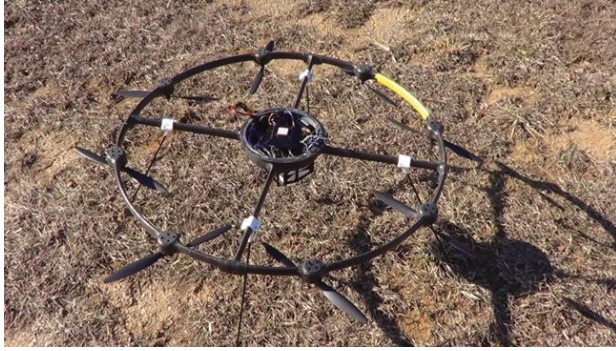
Figure 11. Example airframe constructed using novel additive manufacturing techniques.
