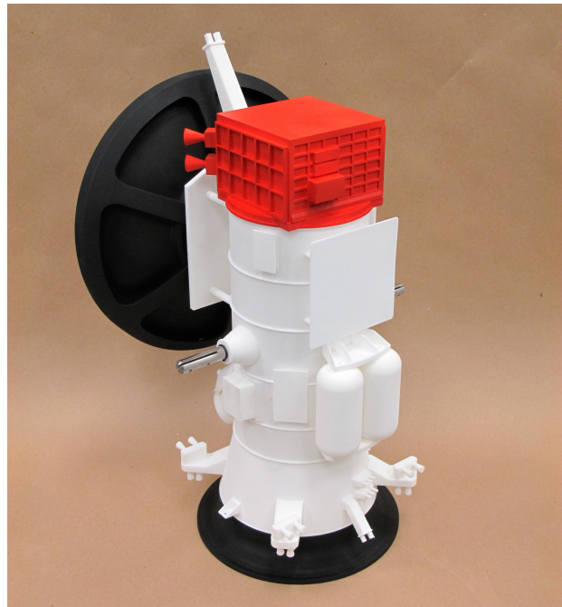
Figure 14. Main structure of EUROPA satellite scale model. The white main body was made with glass-filled nylon on a powder bed fusion AM system, and the black and red sections were made out of ABS thermoplastic on a material extrusion system.
