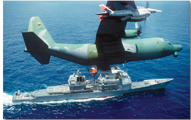
Figure 12. Still used today, two Teledyne-Ryan AQM-34 drones are carried on the wings of a DC-130 Hercules aircraft.
