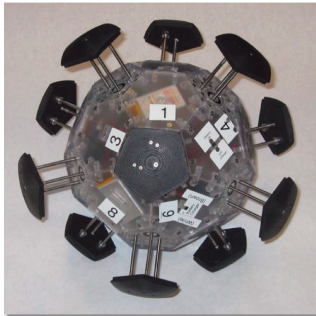
Figure 1. Image of Buckybot with all 12 of its actuators extended.
