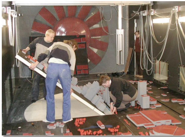
Figure 4. View of the 4 × 3 m test section at the University of Hamburg wind tunnel as a section of the Oklahoma City model is being put in place. A turntable is used to allow consideration of different wind directions. The scale is 1:300. (Reprinted from Ref. 7 with permission of the American Institute of Aeronautics and Astronautics.)
