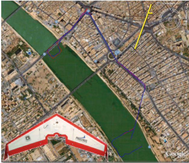
Figure 9. Illustration of the Procerus Unicorn UAS and the notional mission route through downtown Baghdad with winds from 020° at 3 m/s. (Adapted from Ref. 7 with permission of the American Institute of Aeronautics and Astronautics.)
