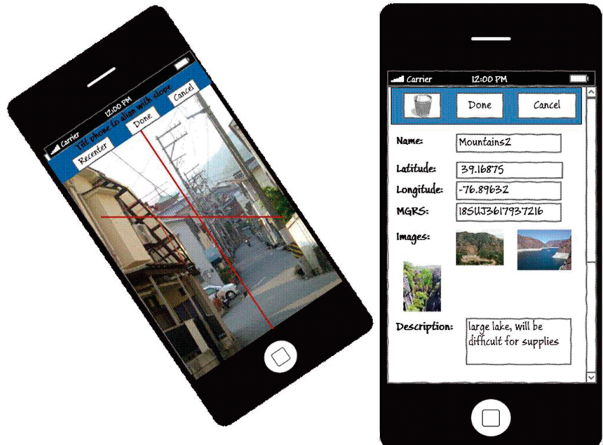
Figure 6. Screens from the data collection app, which were included in a mock-up built using Microsoft's Expression Blend and SketchFlow tool. The angle-measuring tool (left) estimates the slope of an object in an image. Data about a particular point of interest, including geo-tagged images, are shown on the right.
