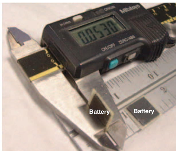
Figure 4. Photograph of two 1-cm 2 , 53- \mu m-thick polyurethane batteries.
