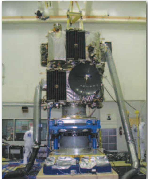
Figure 3. Stacked STEREO observatories on the APL vibration table.
