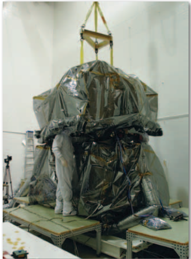
Figure 12. Contamination preparations for acoustical testing at GSFC.
