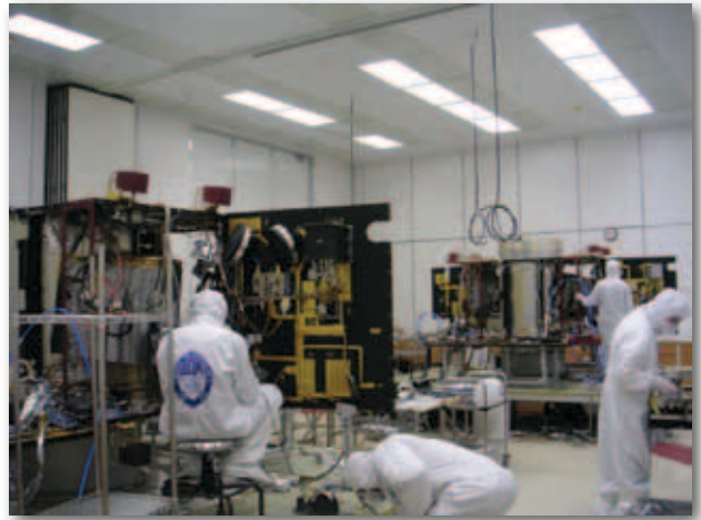
Figure 8. Spacecraft A (foreground) and Spacecraft B (background) with panels splayed open during component integration in the APL cleanroom.
