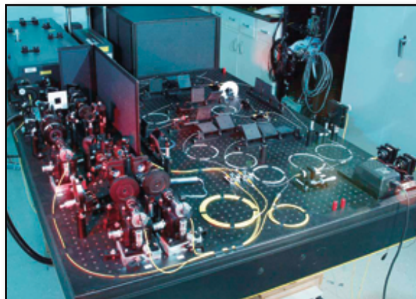
Figure 12. Experimental apparatus used to demonstrate the first quantum controlled-NOT logic gate for single-photon qubits.
