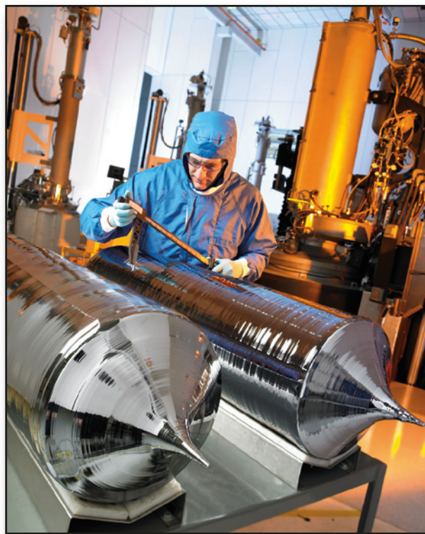
Figure 3. Photograph of as-grown 300-mm-diameter silicon ingots with a Czochralski puller in the background. (Reproduced with permission from MEMC Electronic Materials, Inc.)
