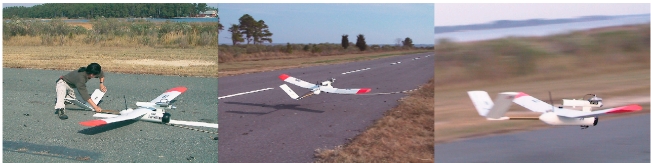
Figure 3. (left to right) Preparation for launch, launch, and landing of the L3-BAI Aerosystems Javelin.
