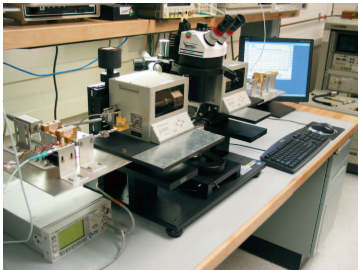
Figure 2. The APL load pull measurement system allows characterization of RF transistors into variable fundamental and harmonic loads. (DUT = device under test, F_0 = fundamental frequency, GPIB = general-purpose interface bus, I_{ds} = drain-source current, I_{gs} = gate-source current, Iso = isolator, PA = power amplifier, V_{ds} = drain-source voltage, and V_{gs} = gate-source voltage.)
