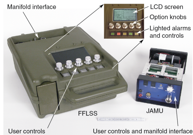
Figure 1. Images of the FFLSS and the JAMU. The FFLSS is shown packaged in its final configuration. In the inset image, note the functional graphic display and the illuminated controls. The JAMU, shown without its outer shell, is a considerably smaller ventilation unit.
