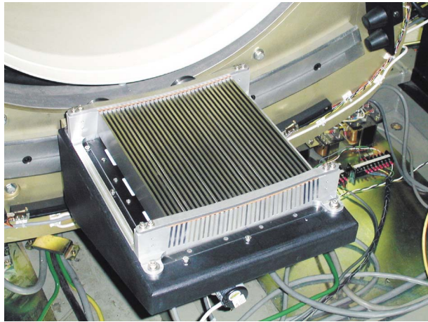
Figure 9. Photograph of the high-performance antiscatter grid mounted over the flat panel detector of the HTB.
