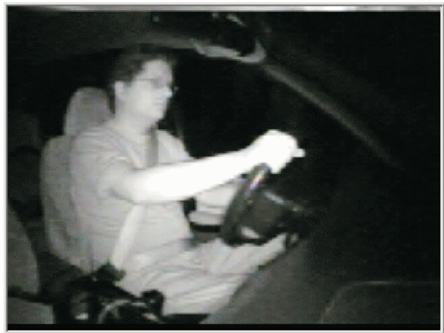
Figure 1. Images captured on a street with no lighting at about midnight. Traffic conditions were recorded using a low-light-level monochrome camera (left). An image of the vehicle operator was recorded with a monochrome camera with an integrated infrared light emitting diode illuminator (right).
