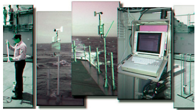
Figure 3. SEAWASP environmental assessment subsystems include rocketsondes, ship topside environmental sensors, and computer programs to assess radar performance capability.
