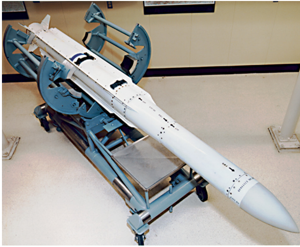
Figure 1. Evolved Seasparrow Missile. The kinematic improvement of the ESSM adds a 10-in.-dia. rocket motor that can be launched from all consortium launching systems and can fit four to an Mk 41 VLS cell. Missile guidance options and an improved warhead provide additional capabilities for this newest self-defense weapon.
