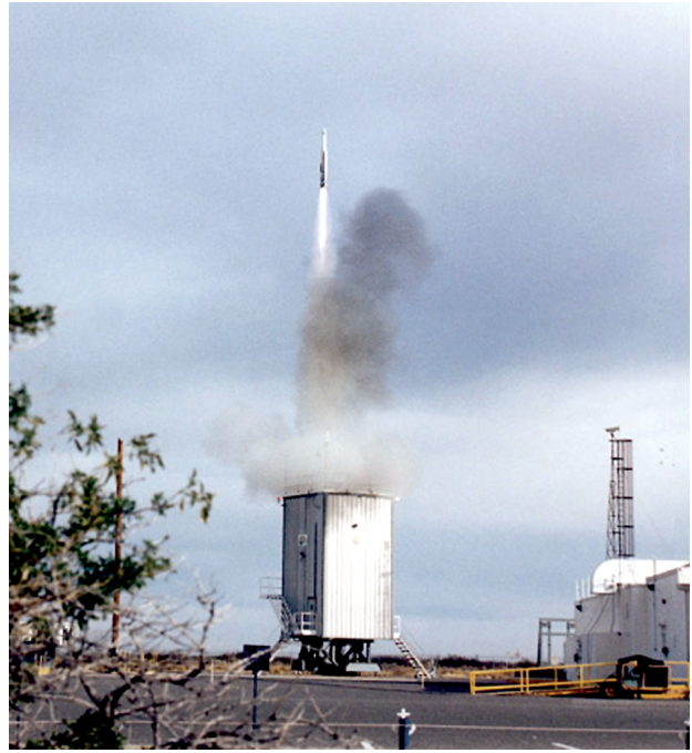
Figure 2. Controlled Test Vehicle 3. The ESSM is launched from an Mk 41 VLS in a quad-pack configuration. This will be the primary launching system for ESSM aboard several consortium ships, including Aegis.
