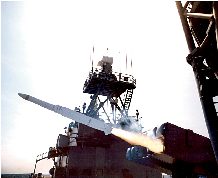
Figure 5. ESSM firing from the Self-Defense Test Ship. This was the first at-sea launch of ESSM from an Mk 29 trainable launcher aboard the SDTS. It was also the first of a series of at-sea developmental and operational firings of the ESSM following a successful CTV/GTV test program.
