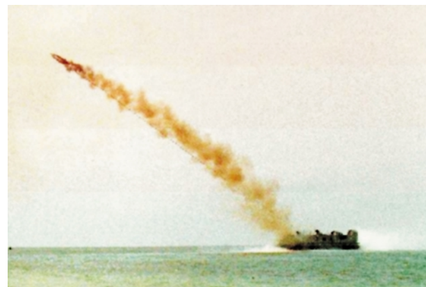
Figure 3. LCAC firing a SABRE line charge into the surf zone. A special autopilot has been designed to facilitate this capability. One LCAC can carry a combination of SABRE and DET systems.
