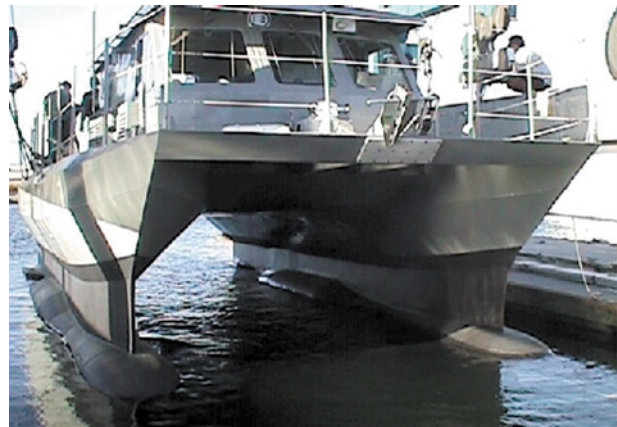
Figure 5. The 41-ft SWATH vessel currently operated by Explosive Ordnance Disposal Mobile Unit 7 provides a stable platform through Sea State 3 for searching and prosecuting mines. This one is sized to fit inside a C-5A aircraft.
