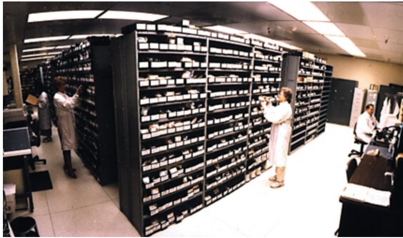
Figure 2. The staging area for flight-ready electronic parts currently holds over 1 million piece parts with a purchase cost of over $12M. The inventory is managed using a commercial Manufacturing Resources Planning (MRP II) system, MFG/PRO.
