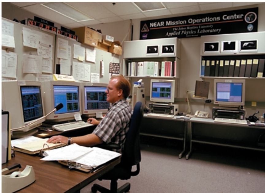
Figure 3. NEAR Mission Operations Center in the real-time control pit. The flight controller interfaces with a three-monitor display system to keep track of all operations.
