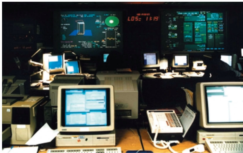
Figure 5. MSX Mission Control Center showing the DataViews and SeeMSX overhead displays that enable very fast real-time assessment of the spacecraft's health. It allows flight controllers to quickly move from assessment to the command loads and tape recorder playbacks. Speed is critical in low-Earth-orbit missions where contacts only last about 10 min.
