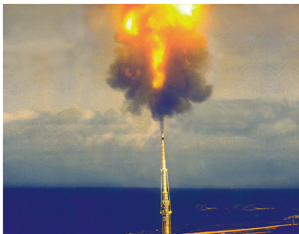
Figure 1. Firing of the 16-in. HARP gun in Barbados. In the late 1960s and early 1970s, the gun was used to launch rockets as well as scramjets at muzzle velocities up to 1.6 km/s.
