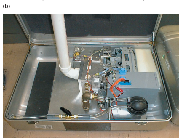
Figure 5. Aerosol impactor collector. (a) Movement of air flow. (b) The portable unit is linked by an RS-422 to a remote notebook computer that provides monitoring and high-level commands.
