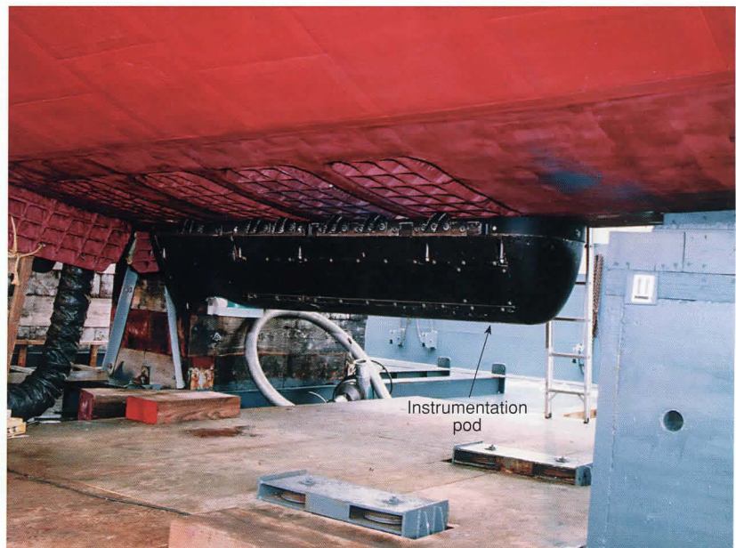
Figure C2. Ocean Data Acquisition Program external instrumentation pod affixed to the bottom of a submarine in drydock.
