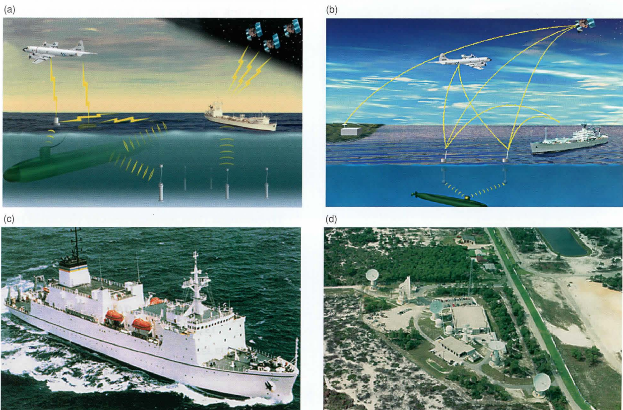
Figure A3-2. Launch area portable range instrumentation. (a) The submarine Buoyant Cable Communications System (BCS) is used for two-way communications with the launch area support ship (LASS), and (b) the Portable Underwater Reference System provides real-time submarine position determination. The Flight Test Support Systems (c) on the LASS (USNS Waters ) and (d) at the Jonathan Dickinson Missile Tracking Annex Down-Range Support Site ground station provide the eastern Range Command and Control Center at Cape Canaveral, Florida, with real-time data for range safety purposes.
