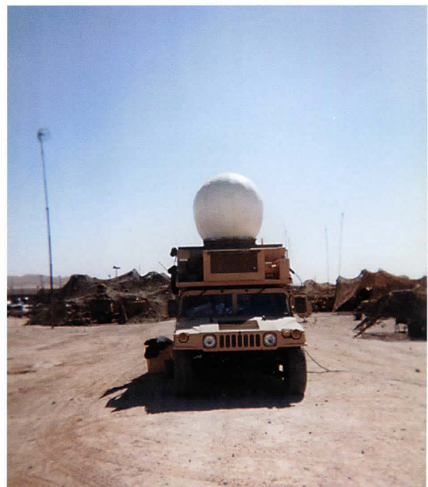
Figure B2-4. APL-developed UAV Tactical Control System stabilized pedestal and antenna mounted on an Army high-mobility multipurpose wheeled vehicle.
