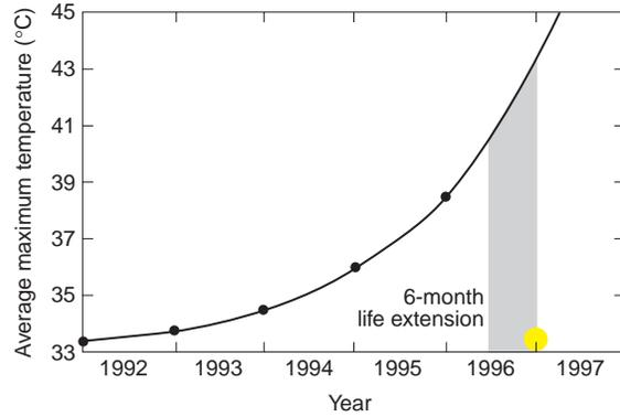
**Figure 15.** Plot of winter full-Sun seasonal average battery temperature for Nova 2. A significant reduction of battery temperature resulted from using the 11-cell voltage/temperature curve in 1996. The yellow circle indicates the actual temperature point. This temperature reduction increased the satellite lifetime by at least 6 months.
