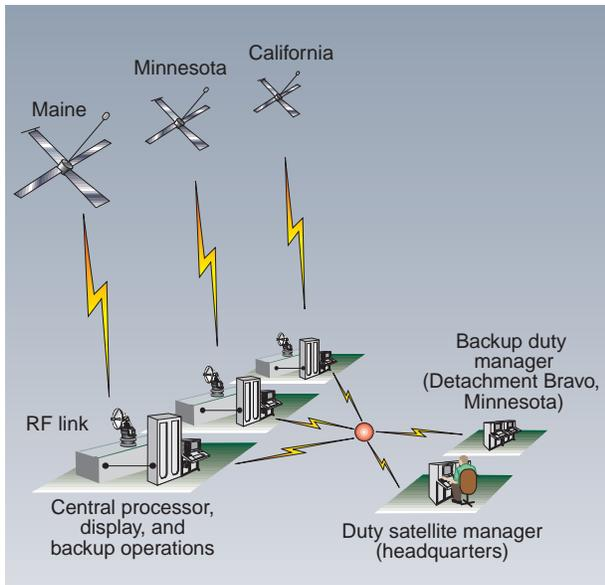
**Figure 8.** The duty satellite manager at headquarters normally controls all operations. A duty manager at the backup site assumes controls if headquarters is disabled.
