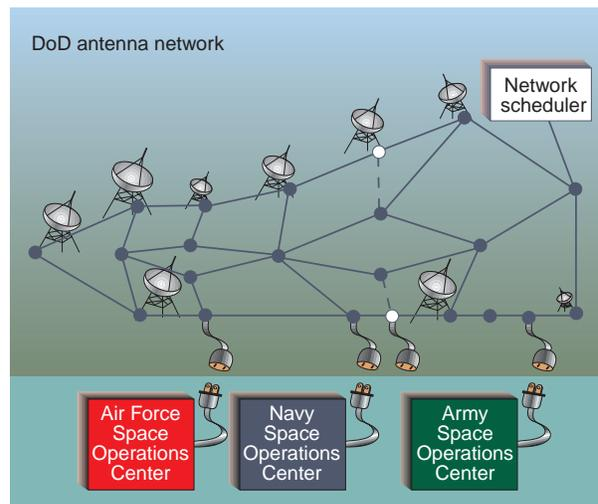
**Figure 2.** Diagram of the “plug n’ use” concept of satellite control. NAVSOC “plugs” into Air Force Satellite Control Network sites via Falcon Air Force Base to control Fleet satellites.
