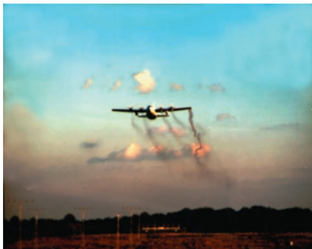
Figure 9. The C-130 with trailing vortex on approach to BWI.
