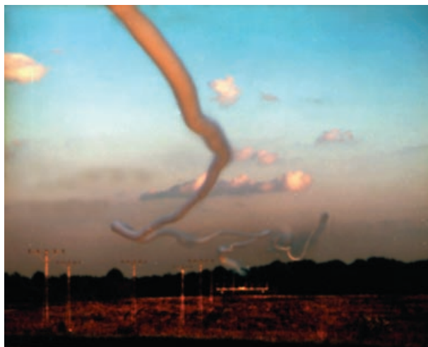
Figure 10. Smoke-marked vortex as seen several seconds after the C-130 passed by (Fig. 9).
