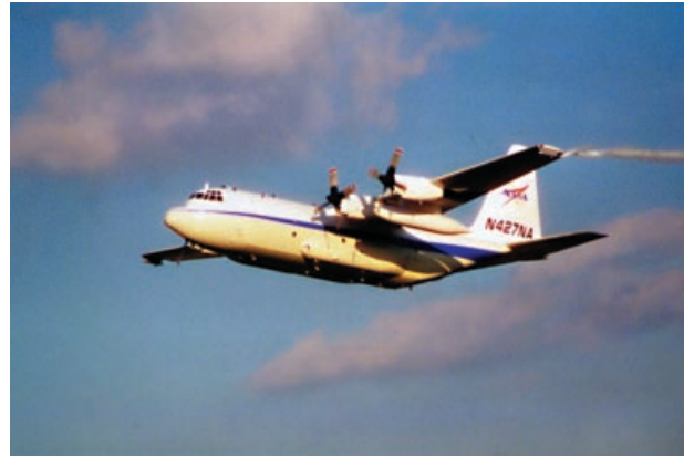
Figure 8. A NASA C-130 research aircraft with smoke generator on left wing tip.
