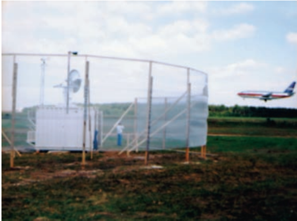
Figure 7. Wake vortex receiver site at BWI airport.
