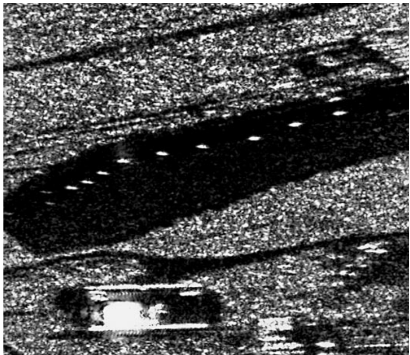
Figure 5. The uncorrected SAR image. The image contains 12 reference radar reflectors, only 9 of which are clearly visible. The visible targets show significant azimuthal blurring.
