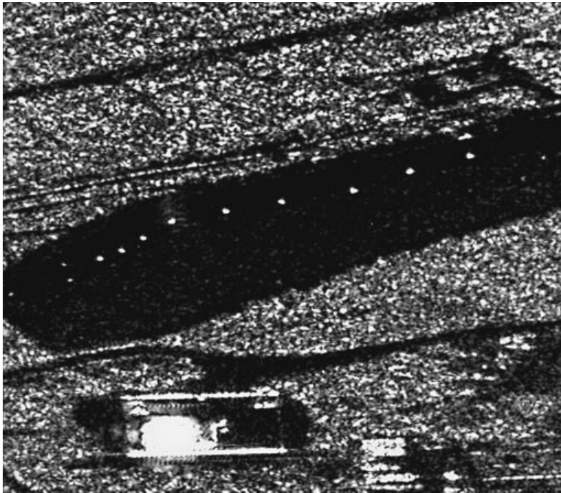
Figure 6. The corrected SAR image. The image contains 12 reference radar reflectors. Note that the targets are well defined. The clutter in the lower right-hand corner is well defined, also.
