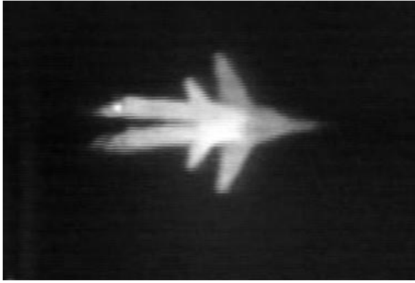
Figure 12. An IR image projected with a resistive heater scene projector. (Photo provided courtesy of Alan Pritchard of British Aerospace's Sowerby Research Center.)
