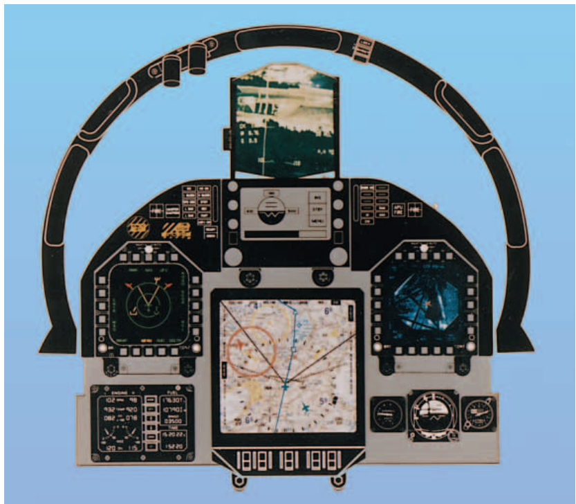
Figure 2. An early rendition of the crew station display for the new F/A-18 E/F. The multipurpose color display is prominent in the center of the picture.
