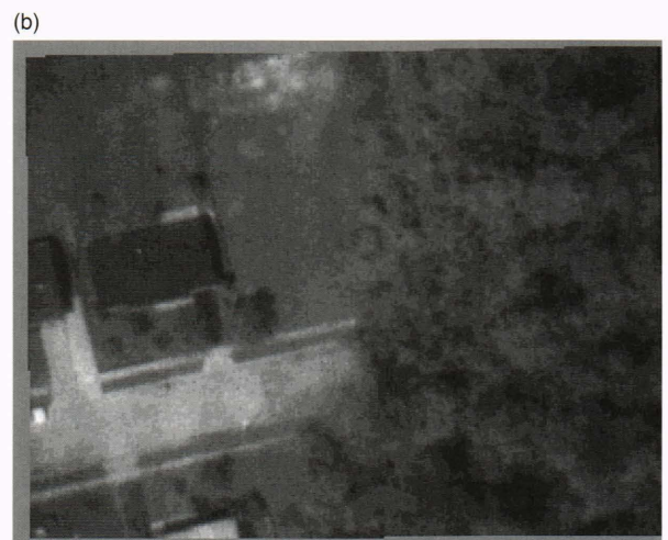
Figure 6. A gray-scale video frame from DSMAC during flight. (a) Original, uncorrected frame; (b) frame corrected to remove geometric errors.
