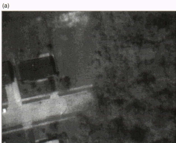
Figure 6. A gray-scale video frame from DSMAC during flight. (a) Original, uncorrected frame; (b) frame corrected to remove geometric errors.
