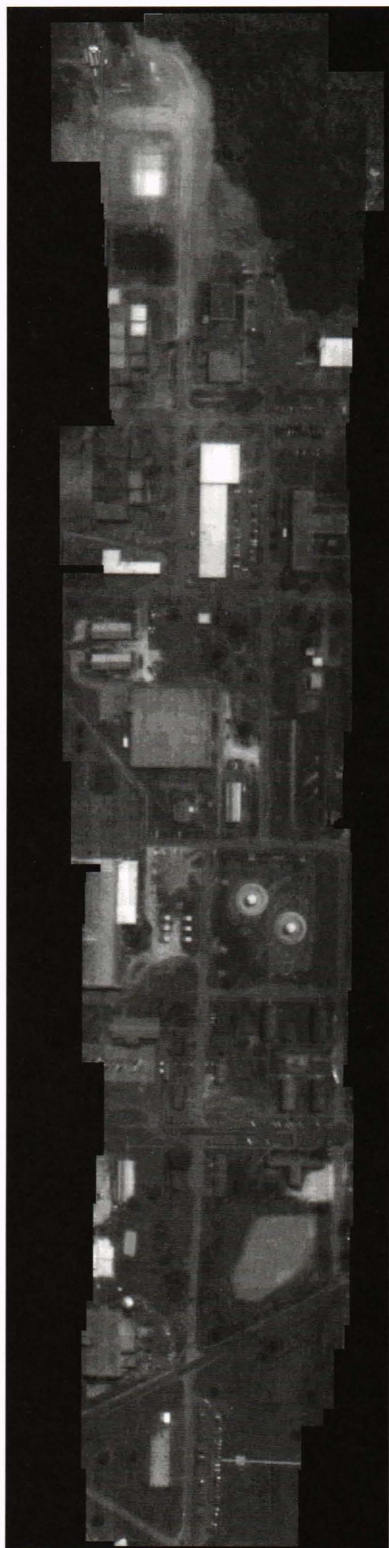
Figure 8. A gray-scale mosaic of DSMAC frames from a test flight. Individual sensed frames are geometrically corrected and pieced together to form the mosaic image.
