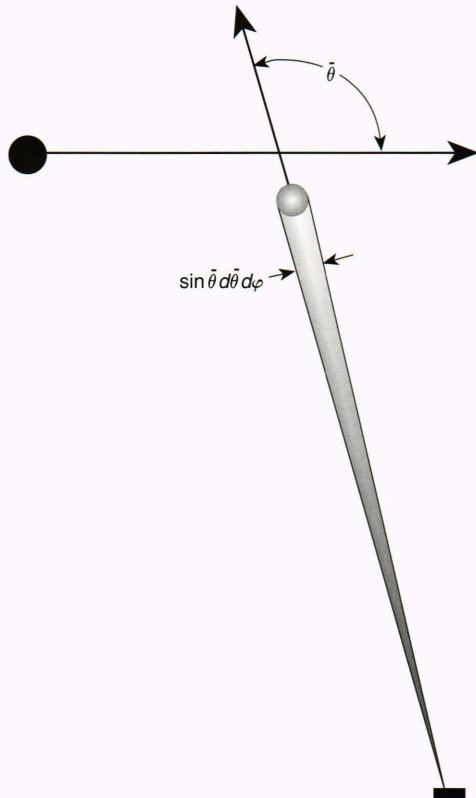
Figure 1. Schematic of a molecule (gray circle) leaving a satellite and encountering an ambient atmospheric molecule (black circle). The angle between the velocity vectors is \bar{\theta} .
