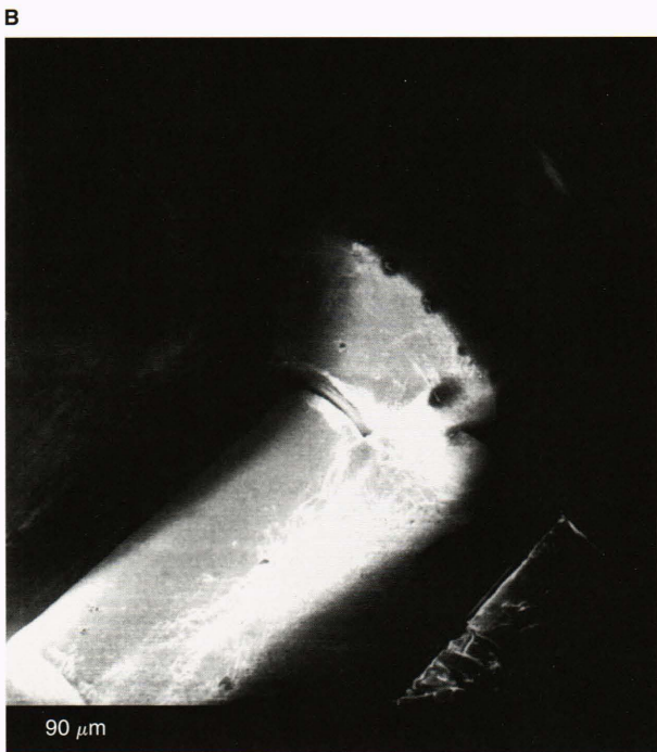
Figure 7. A. Diagram of a tapered launch pin designed to avoid the disadvantages of the flat-tab launch pin. The design improved connector performance only marginally. B. Scanning electron microscope photograph of a fractured pin, taken using a 20-kV electron beam at a 30° tilt. C. Enlarged view of the rift shown in B, taken at the same electron beam settings.
