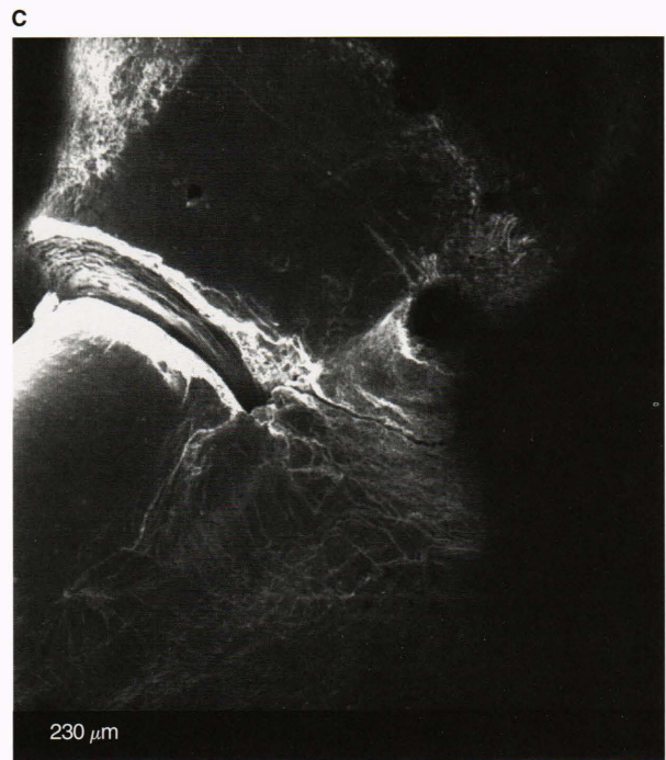
Figure 7. A. Diagram of a tapered launch pin designed to avoid the disadvantages of the flat-tab launch pin. The design improved connector performance only marginally. B. Scanning electron microscope photograph of a fractured pin, taken using a 20-kV electron beam at a 30° tilt. C. Enlarged view of the rift shown in B, taken at the same electron beam settings.
