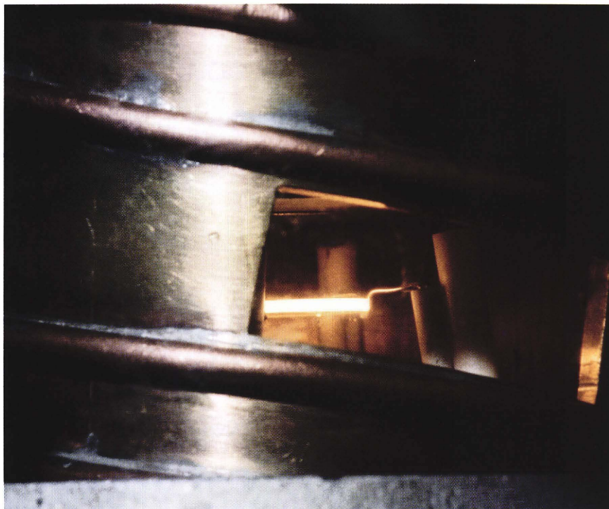
Figure 9. Photograph of a glowing sapphire sample at 1900 K.
