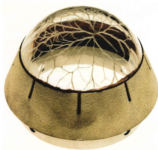
Figure 6. Hot-pressed spinel infrared dome after aerothermal test at Mach 4.6. Total pressure was 900 psia and total temperature was 2500°R.
