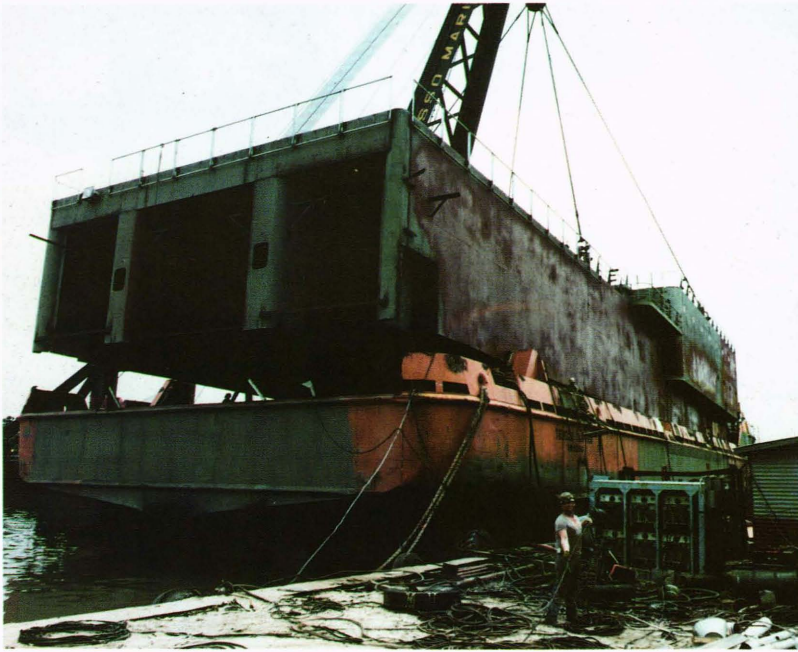
Figure 12. The R/V Cory Chouest . Under contract to APL, Edison Chouest Offshore of Louisiana purchased the M/V Tender Clipper , a Norwegian North Sea pipe carrier. In just four months, APL and Chouest transformed this platform into the most advanced ASW research and development platform in the world. The aft deck was outfitted with engineering, instrumentation, and berthing spaces by the addition of the "APL module" (top). The finished vessel was then reflagged and renamed the R/V Cory Chouest (bottom).
