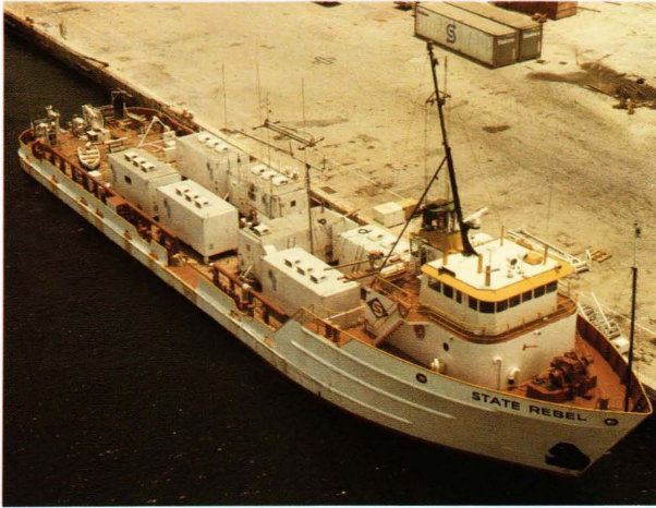
Figure 5. The supply vessel State Rebel , outfitted with vans to provide work space. Extensive measurements of ocean hydrodynamic processes took the Submarine Technology Division to sea in the mid-1970s to mid-1980s. Long-term tests using sophisticated profiling and towed instrumentation to measure conductivity, temperature, and velocity fluctuations made it necessary to outfit large offshore supply vessels with vans for scientists, engineers, and analysts to work in for extended periods of time.
