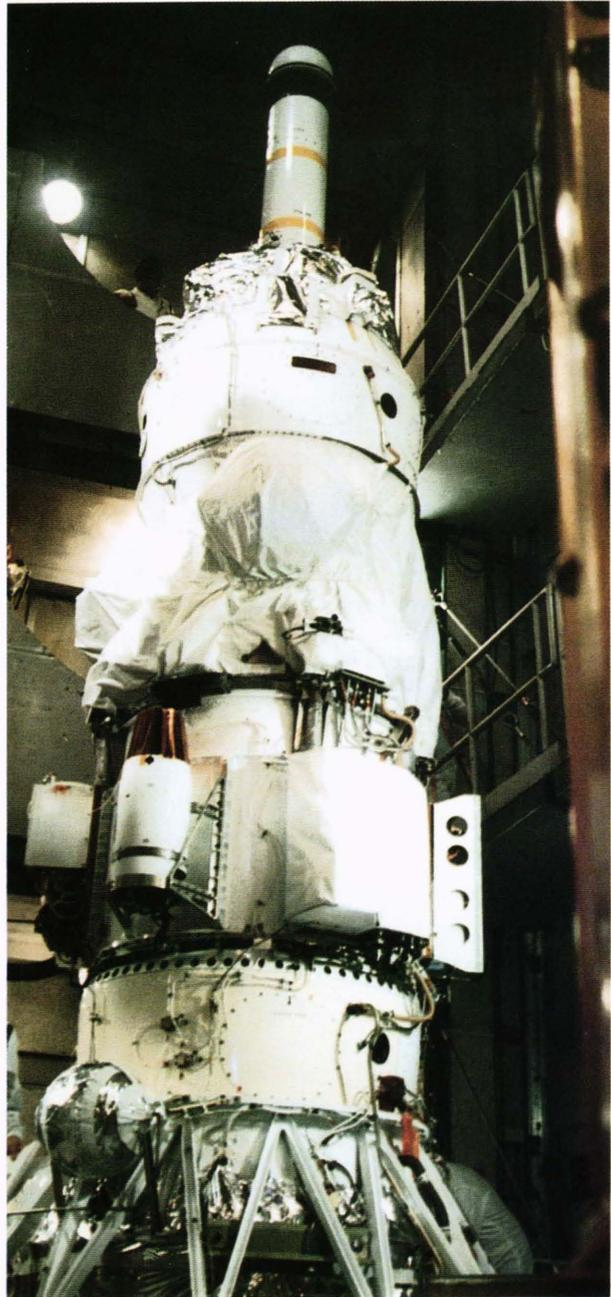
**Figure 9.** The Delta-180 payload being readied for launch on a Delta rocket at Cape Canaveral. The APL-provided payload is shown just beneath the thermal blankets.
